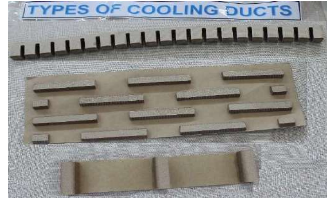
Types of Cooling Ducts
